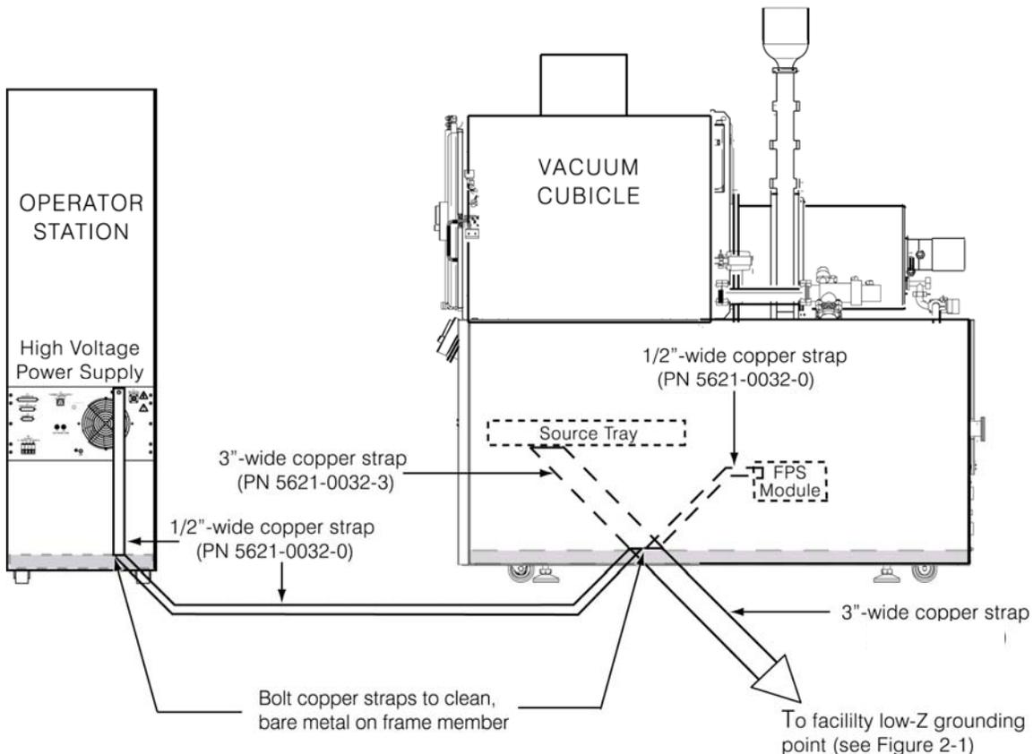
Where copper straps are attached to frame members, the copper must be bolted to clean, bare patches of metal. The length of copper strap connected to the source tray must be securely bolted to a clean site on that part. The upper grounding stud on the FPS module must be connected to the vacuum cubicle's central low-Z grounding point by a length of 1/2"-wide copper strap (thickness: 0.035"–0.050"). The green #10 AWG wire grounds the lower FPS grounding stud to the vacuum cubicle's frame.
