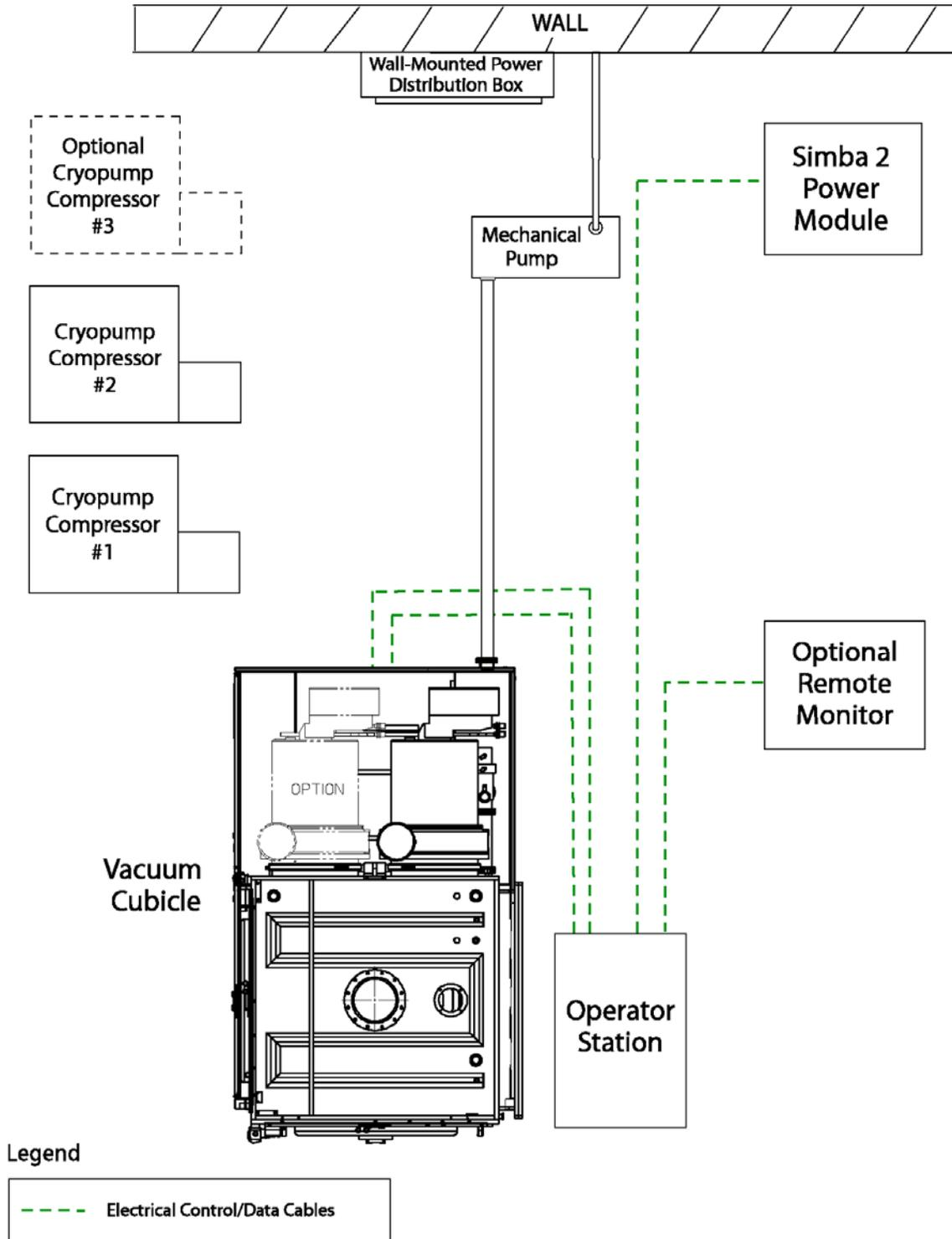
Figure 3-8 Routing of Electrical Power Cables on Simba 2-Powered Systems
