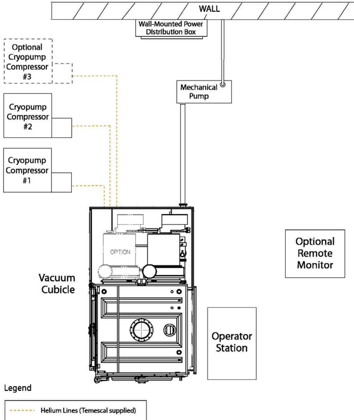
Figure 3-7 Routing of Control/Data Cables on Simba 2-Powered Systems with the Optional Simba 2 Control Console
