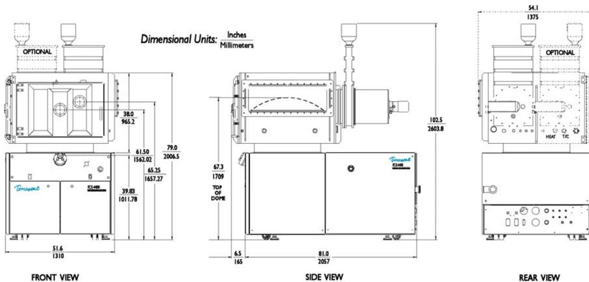
**Figure 3-2 System Plan View, Showing Dimensions of Main System Components (System Shown with Optional Simba 2 Power Supply)**
